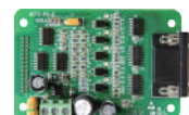
MCTC-PG-D Quadrature incremental encoder card 5 Vdc supply, female 15-way D-type connector (A, A, B, B', 0V @ 5V HTL)
