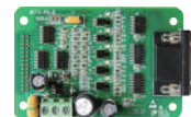
MCTC-PG-D Quadrature incremental encoder card (A, A, B, B') with UVW commutation signals 5 Vdc supply, female 15-way D-type connector
