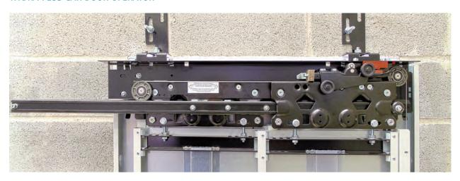
Hydra car door with Wittur PLUS brushless permanent magnets synchronous motor (PMSM) offers the latest technology available on the market. Designed for low power consumption during operation and standby, Hydra PLUS with ECO+ offers a power consumption reduction up to 48% compared to previous drive designs.
